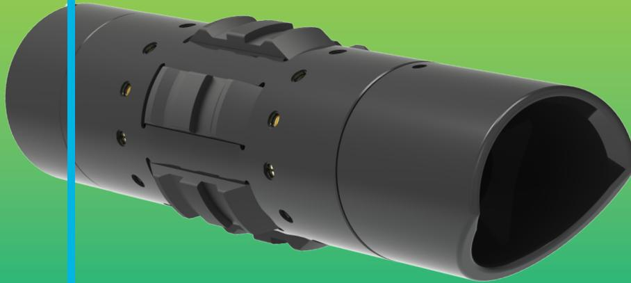
The Stinger shifting tool uses bidirectional key sets to enable single-trip opening and closing of downhole valves and sleeves. Because the key sets are bidirectional they do not require modifications to shift tools open and closed, helping operators to reduce downhole trips, accelerate operations, and minimize OPEX.
